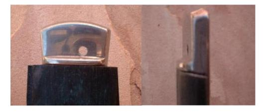
Allright...using any flat belt sander ..make the bevel at the top of both handles it could take a few trys..just go slow and check it often....push the handle up against the bolster and once you like the fit and have no large gaps or light shining through you are ready for the next step which I should have posted later today
