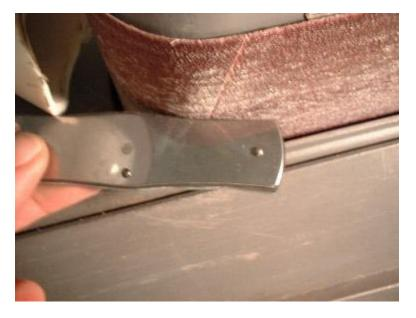
put your handle material back on the liner...put your pins back in and grind as close as you can to the liner
