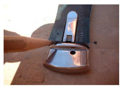
these liners come with a rounded edge...so you know when you have hit it....if you do not like the rounded edge... grind it flat...but don't grind into it too far just yet. When you are done grinding the outline..take a pencil and mark if your material sticks up above the bolster this will give you a guide for shaping the handles
