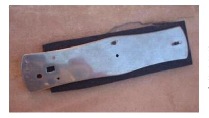
3/32 for the large holes 1/16 for the two smaller ones. As you drill the holes put a pin in each one to keep the material from moving while you drill the next hole. So when you get done you should have your material hanging over the edges of the liners and lots of pins sticking up.
