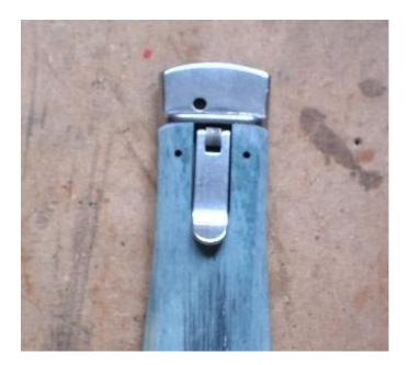
Next take it all apart, and using the line you put at the top of your handle material where you traced around the bolster....shape your handles the way you like. The line helps you make sure they match each other. When you are done take the lever side handle and see how the lever sits
